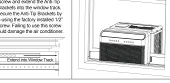
You must extend the Anti-Tip Brackets into the Window
