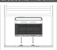
2.1 Set the air conditioner on the support bracket and fold down the side arm hinges.
